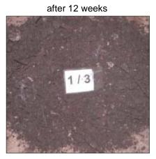
Result: Both fiber types meet the requirements of the disintegration for aerobic composting. The tested nonwovens degraded more than 90 % within a period of 12 weeks.
